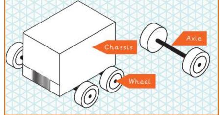
The wheels need to be attached to an axle. The axle needs to fit inside the axle holder but must not be attached to the axle holder otherwise the wheels will not turn properly.
